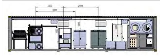
Mobile test rig for electron beam treatment of waste gases and waste water and for plasma-chemical synthesis TABEA
