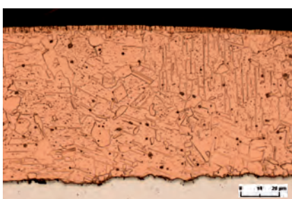
Metallographic cross section of a copper layer
