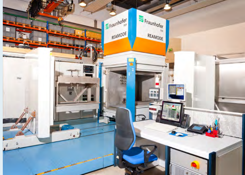
REAMODE electron beam test facility at Fraunhofer FEP
