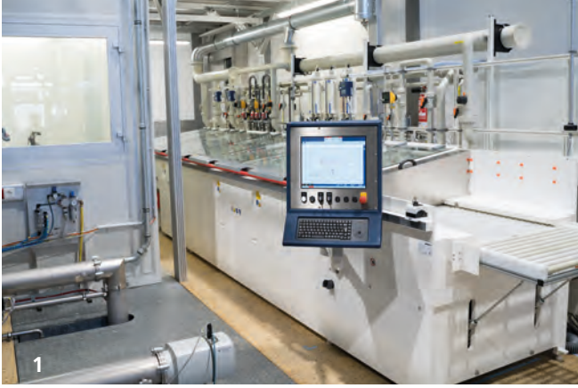
1 Ultrasonic inline wet cleaning line with optimized horizontal roller transport for glass thicknesses from 30 μm to 6 mm (clean room handling in the background)
